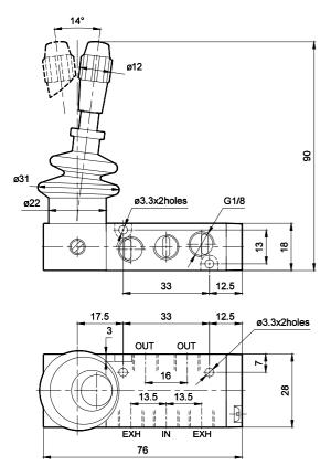
3 / 2 Push Pull operated valve with spring return
